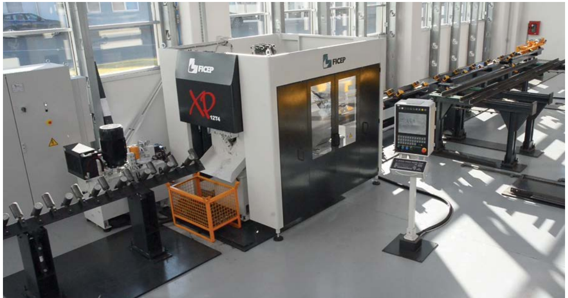
Two XP style angle lines that are clearly the fastest angle lines available on the market today for punching, marking, notching and shearing
